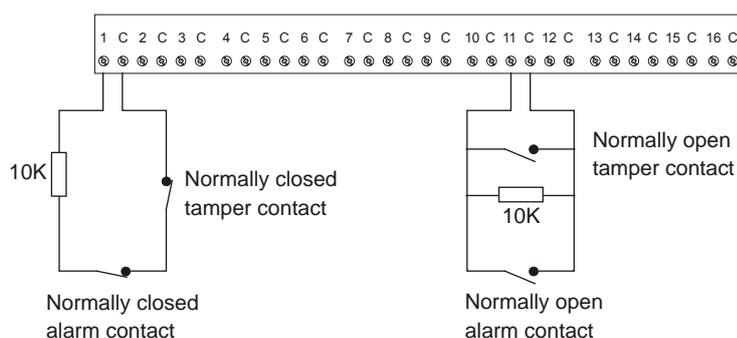
The panel uses the circuit's resistance to determine the state of the zone input:
