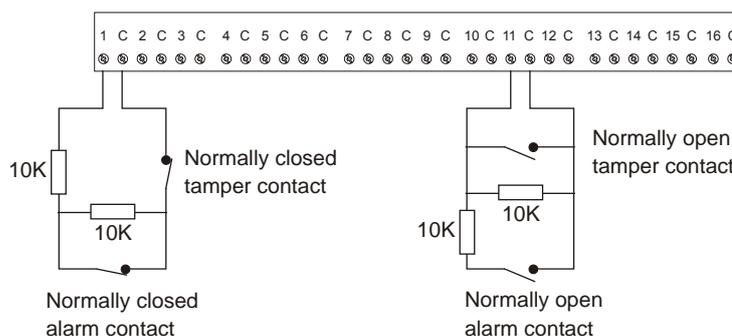
When four-state monitoring is used, the panel uses the circuit's resistance to determine the state of the zone input:
