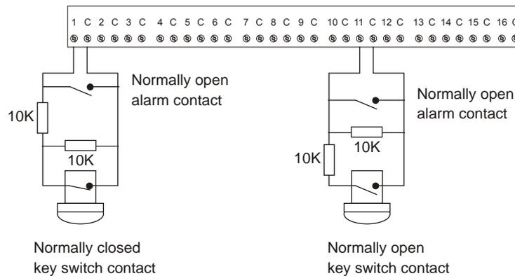
Input type 33 (24-hour alarm & isolate input) is used to wire a key switch and an alarm contact to the same input. For example, a key switch used to isolate a shop's input in a shopping centre where only one input is available for each shop. Alarm is generated when input changes from sealed to open or short.
